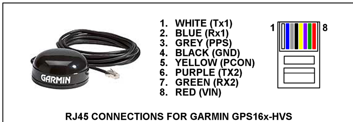
Figure 3: RJ45 Connections for Garmin GPS16x-HVS
